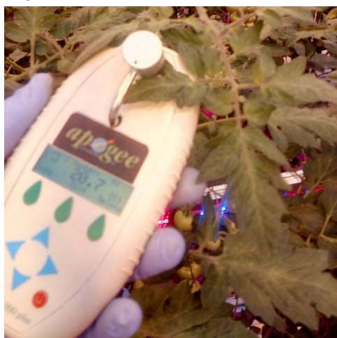
Fig. 2. Measurement of chlorophyll content index in leaf with CCM-200 (left) and bilateral traits of tomato leaf (right)
